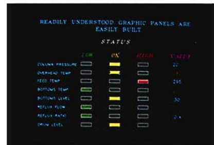
Figure 1. CAMM screen shows graphic panel with acquired data and system status in tabular form.
